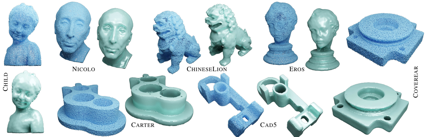
Figure 1: Denoising through line processes. By globally optimizing a robust and regularized fitting energy using line processes associated with local pairs of tangent planes, our method can robustly denoise raw point clouds (blue dots) while leaving features (if any are present) well preserved (green). Denoised pointsets are then visualized via their interpolating reconstruction through advancing front [DCS22] to offer a clearer visual evaluation of their (piecewise) smoothness.
